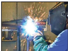
Frames are welded together
